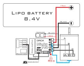
\* Install/Solder the relevant battery connector (Battery Specific) to the battery wires. Red to +ve and Black to -ve. (WARNING! Reversing the battery polarity will destroy your ESC and yoid the warranty.)
