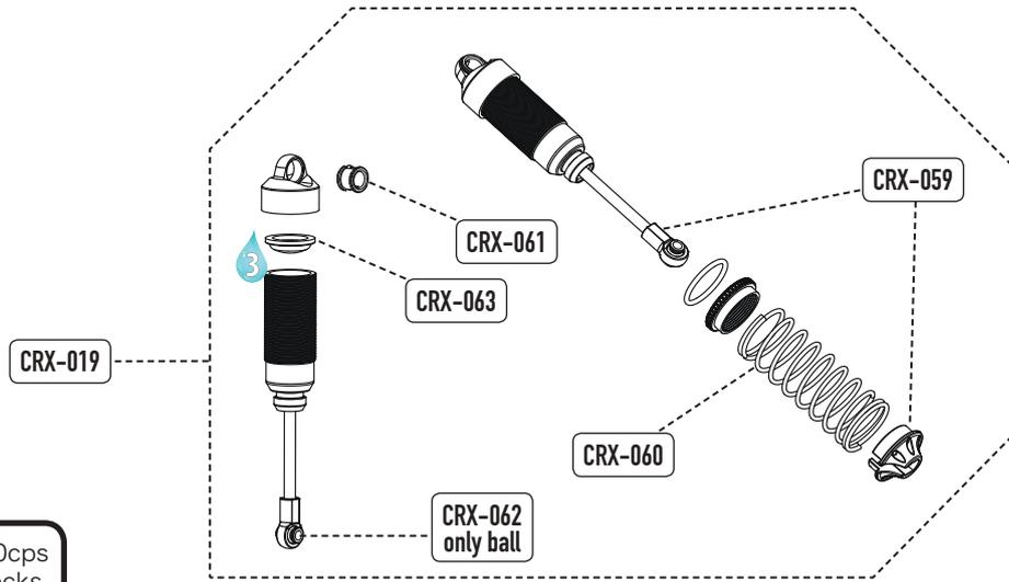
⚠ Use 100cps to 200cps silicon oil to fill shocks
